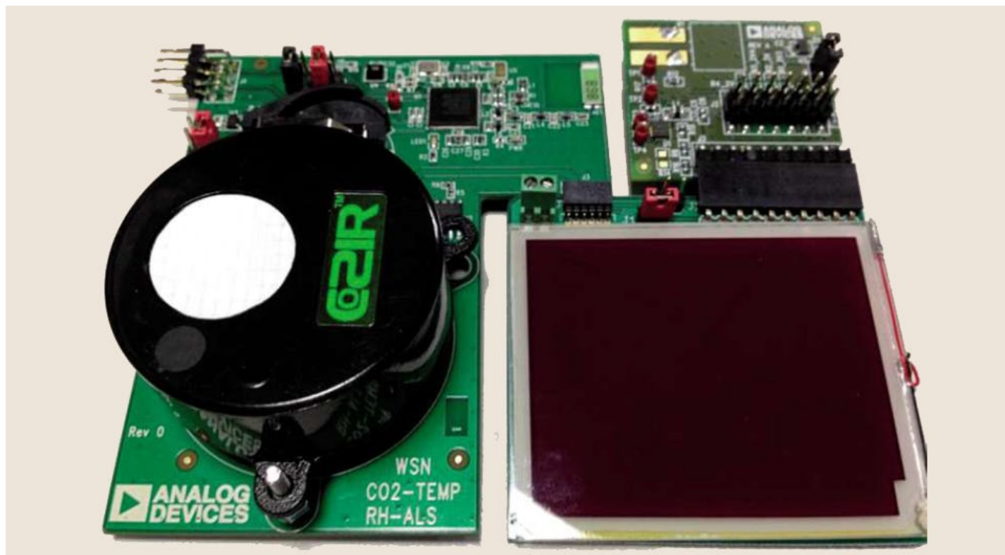
Diagnostic platform based on the ADP5090, with an Ambeon solar panel and CO 2 (Cozir), humidity, and temperature sensors. Not only can it be used for its energy harvesting capabilities, but also as a full system for a diagnostic.
